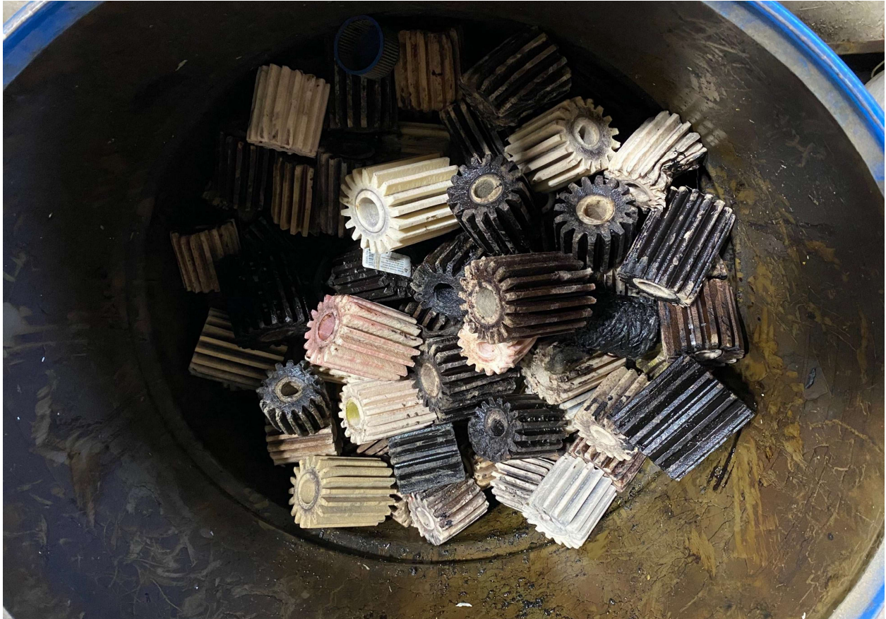
Used cartridge filters in our scrap filter barrel. All filters above from routine annual C&S.
