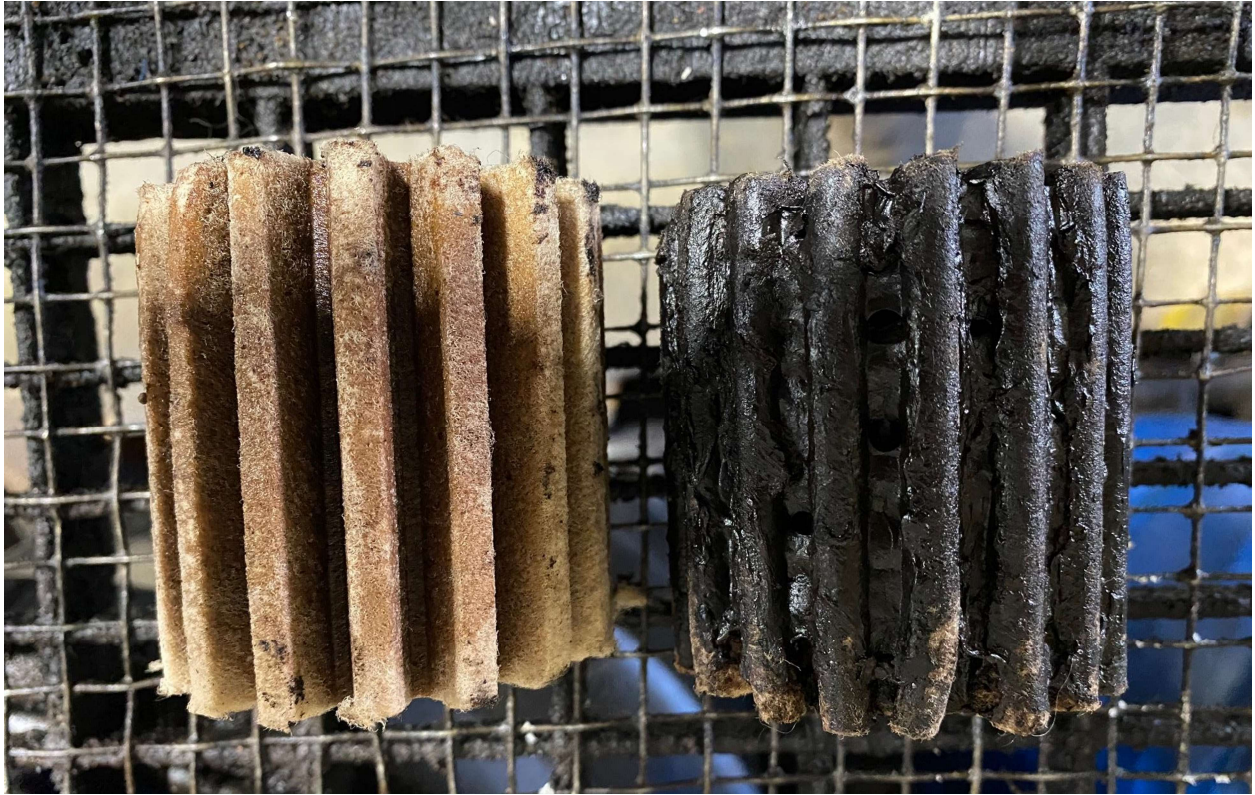
Typical filter from customer using Heating Oil Plus™ vs. biofuel customer in service for one year.
